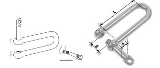
**FIELD OF APPLICATION** Long D-Shackles (removable pin) are designed for appliation where a quick setup with long reach opening are required. Long D-Shackles (collared pin) are designed for application where a more secure tight pin is required.
