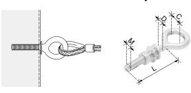
**FIELD OF APPLICATION** Eye bolts (with double layer washing design) are designed for assembly onto a flat panel and serve as a pulling ring.studs for different applications.
