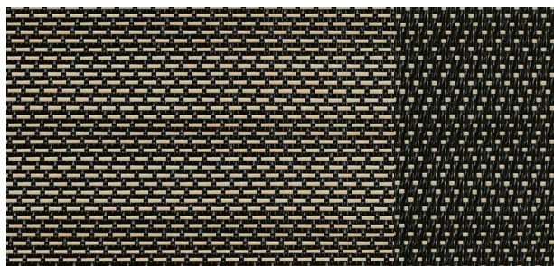
BROKEN TWILL CONSTRUCTION
